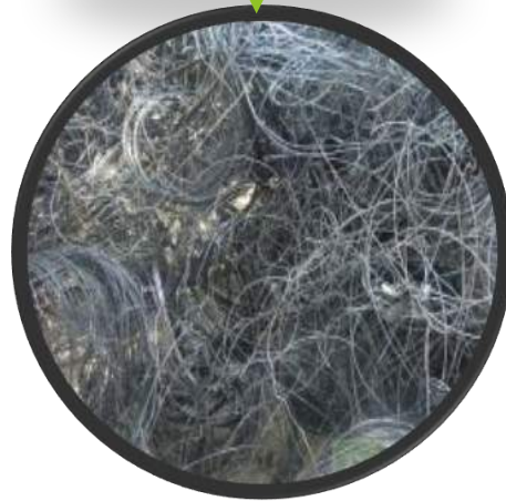
Waste wire in tire
