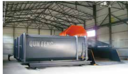
Oslo horizontal compression equipment in Norway
