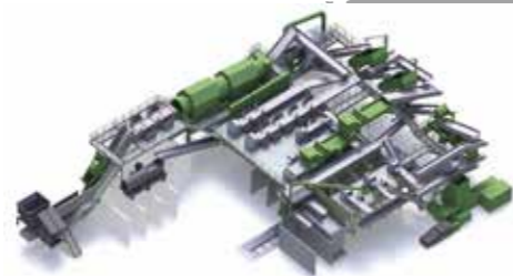
Project drawing of Bulgaria Waste sorting system equipment (300Tons per day)
