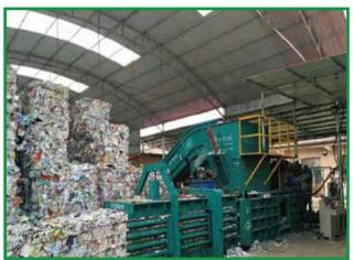
Qunfeng Paper baler machine used for baling press waste paper and similar products with special strapping to form bale, with outstanding performance to reduce the volume, so as to save transportation cost, for the purpose of the enterprise to increase economic benefit.
