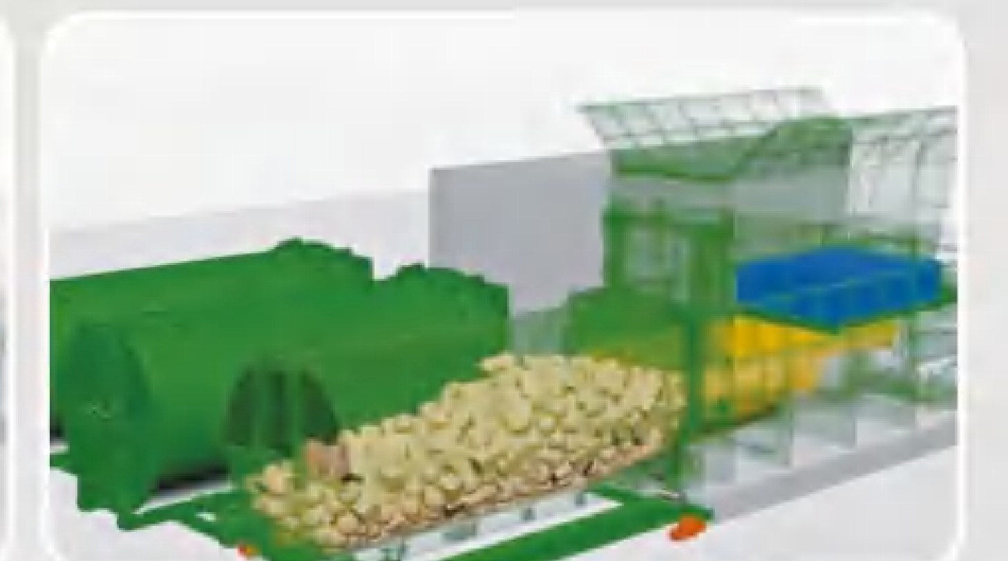
The waste compressed can be reduce to 1.5 times smaller than the original volume to increase the transferring capacity
