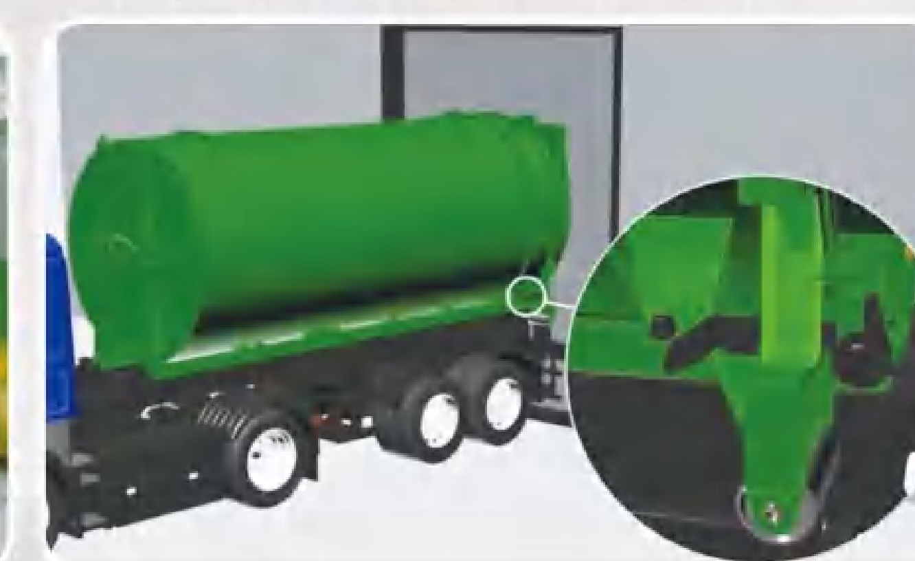
Automatic unlocking of the container cover automatically realize to discharge
