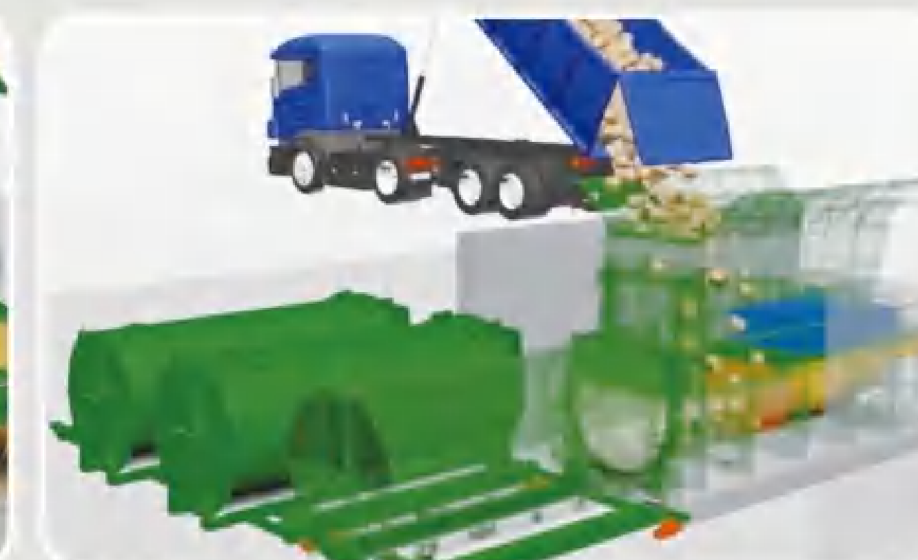
The auxiliary propulsion system moves back to open the discharging hopper; when the hopper is full, the auxiliary propulsion system compresses the waste into the container
