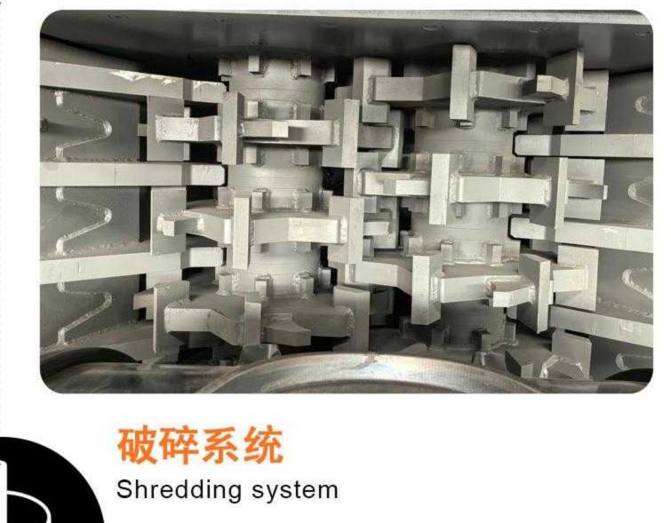
双轴同步破碎系统, 配有可倾斜式料斗 Dual-shafts synchronous shredding system, equipped with tiltable hoppers
