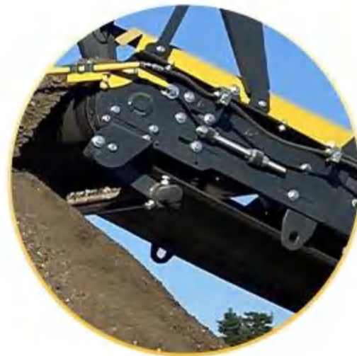
对流向传送带的 出料进行优化 Optimised material flow from the vibro-channel to the main discharge belt
