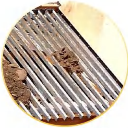
筛网采用常用的条形筛 The screen mesh adopts the commonly used bar screen
