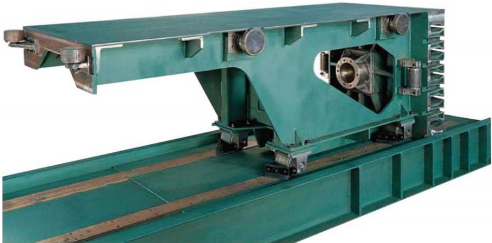
压头上下安装重型滚轮，承受力大，双面有滚轮，减少壁面磨损。均采用易润滑、更换简单的设计。 Heavy-duty rollers install on top and bottom of Ram to bear huge force, double sides have rollers to less wear of wall. All are with designing easy to lubricate and simple replace.
