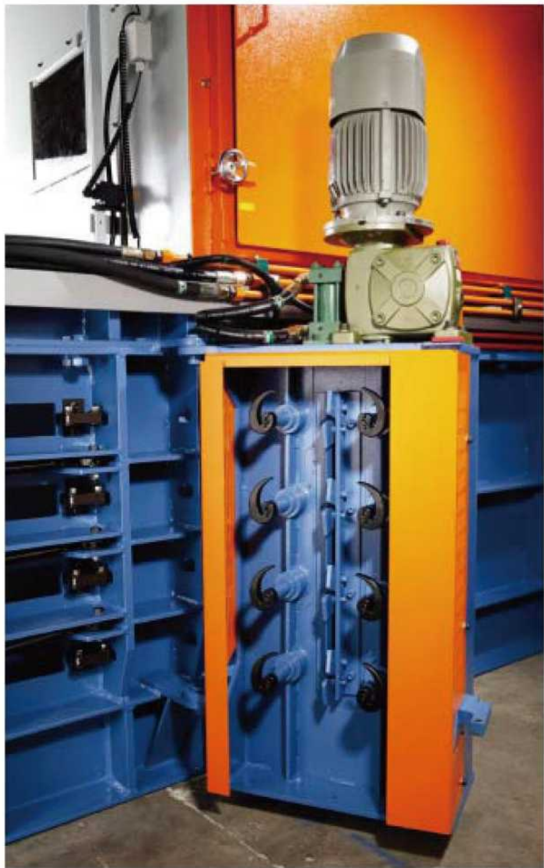
独特的自动捆包装置，提高捆包速度。结构简单，故障率低，易于清洗。 Exclusive auto-tier system increases speed of bale tying. The simple structure is optimum for less maintenance and easy cleaning.
